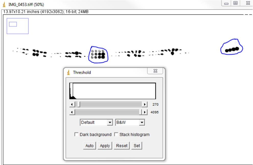
Figure 3: Areas exceeding threshold of 1500 Candela/M<sup>2</sup> (LED fixtures circled in blue)
