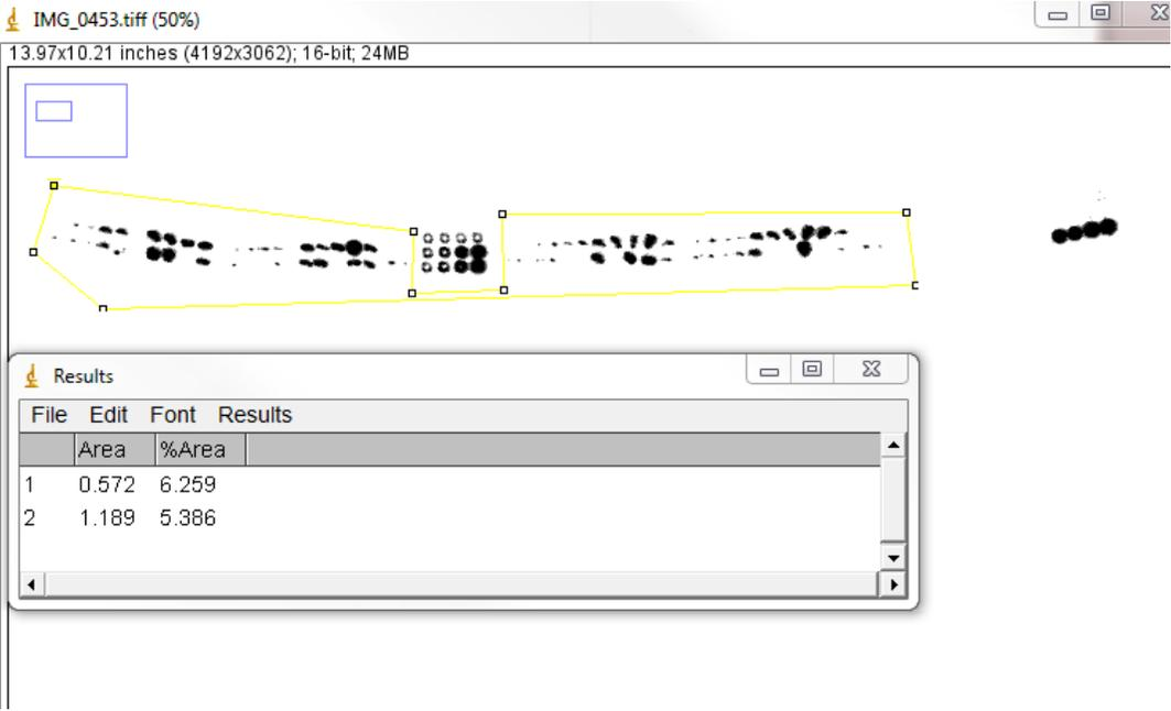
Figure 4: Measuring the Glare Producing Areas
