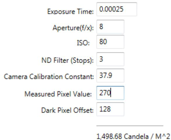
Figure 2: Determining a pixel value limit of 270 for an luminance value of 1500 Candela/M<sup>2</sup>
